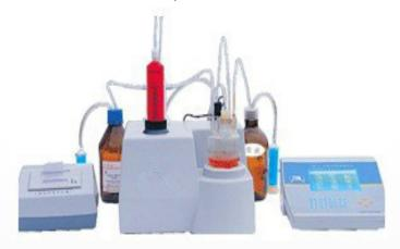
Adopted Karl Fischer volumetric moisture can be measured liquids, solids and gases in the sample crystal water, adsorbed water, free water.
