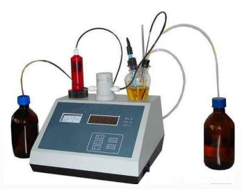
This tester is auto-analyzer used Karl Fischer titration method for the determination of moisture content.
