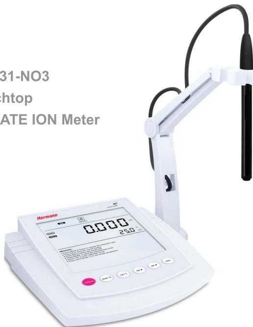
Professional benchtop nitrate ion meter, 5 points calibration, selectable concentration unit. The meter is used for measuring the nitrate ion concentration of samples. Accuracy: 0.5% F.S.
