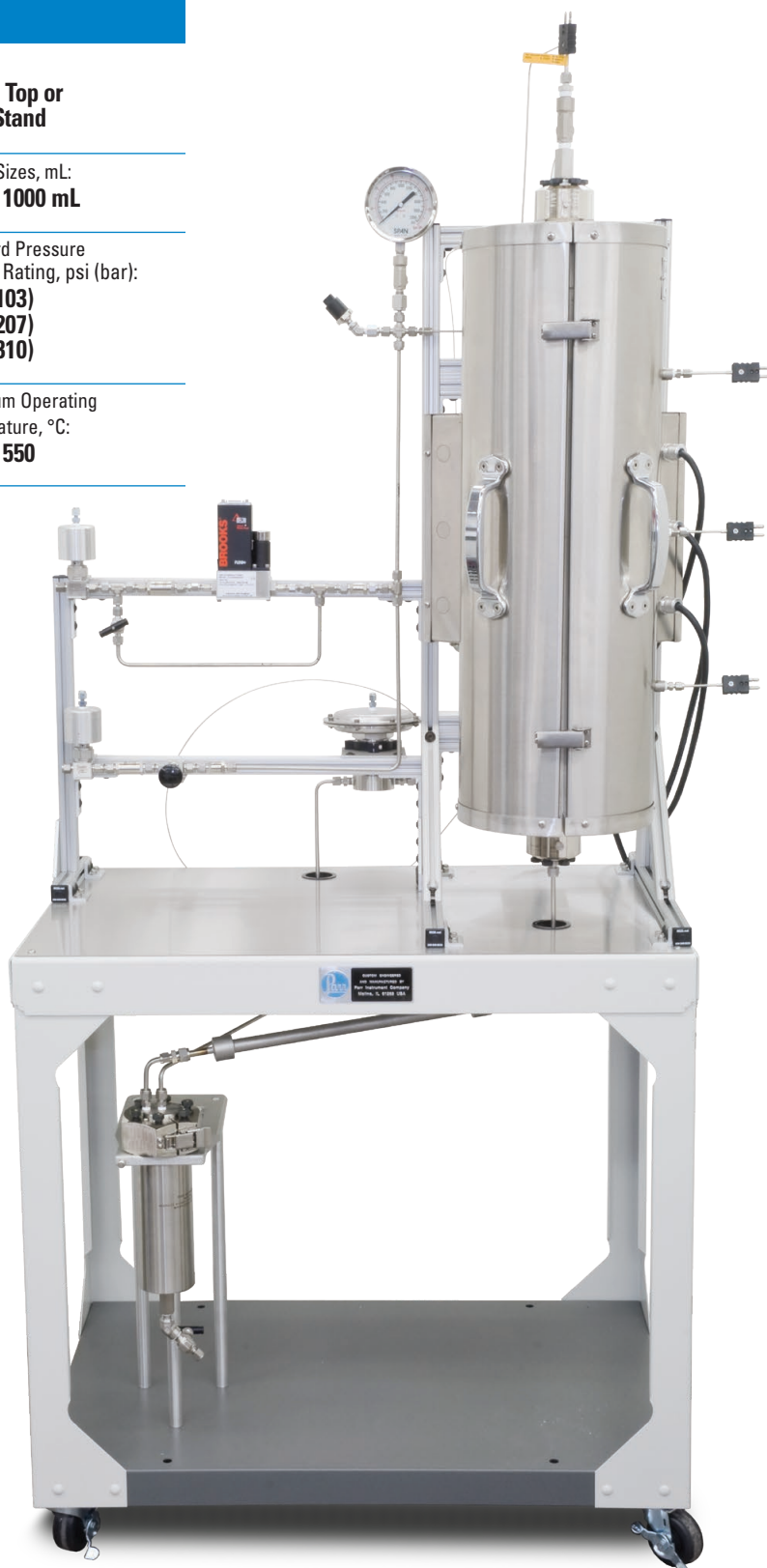
Model 5403 with a 1" inside diameter x 24" length, 3-zone split tube furnace with gas feed system, cooling condenser, and gas/liquid separator vessel.
