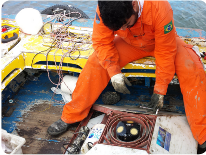
Pyramidal housing protects the Argonaut-XR from damage in busy ports, as shown here in Brazil.*
