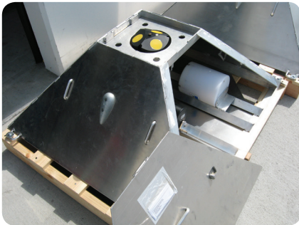
An XR and battery pack installed in an optional trawl-resistant mount.
