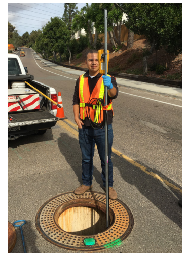
Example of FlowTracker2 used in a storm/waste water pipe.
