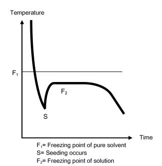
The point "S" is where seeding occurs. Solution freezing point temperature is measured at the plateau.
