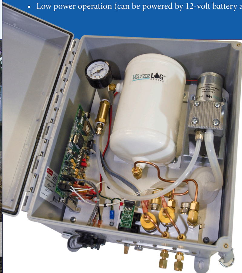
Bubbler System – Photo Courtesy of Grand River CA – Ontario Canada
